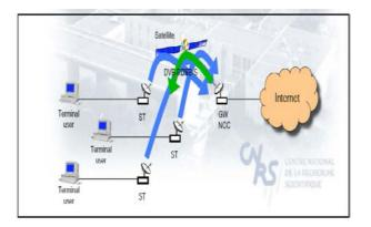
Figure 1: Star topology in Transparent Satellite
