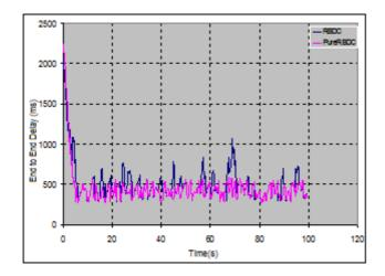
Figure 6: Comparison of two algorithms delay RBDC, Pure RBDC
