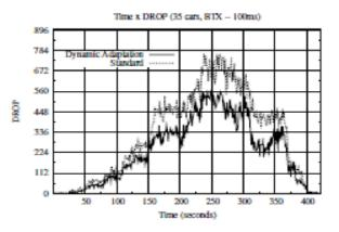
Figure 6: Quantity of overall packet losses for sparse scenarios
