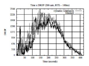
Figure 8: Quantity of overall packet losses for dense scenarios
