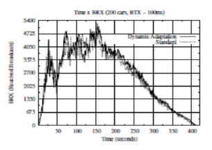
Figure 11: Overall quantity of received packets per second for dense scenarios
