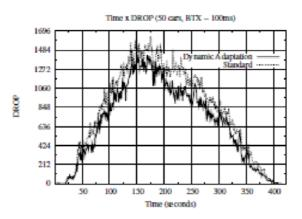
Figure 7: Quantity of overall packet losses for medium scenarios
