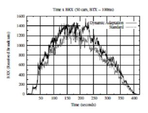
Figure 10: overall quantity of received packets per second for medium scenarios
