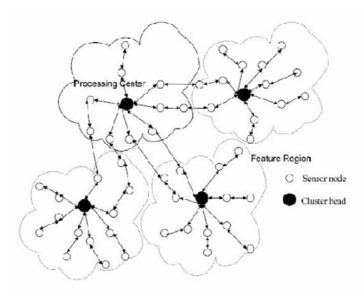
Figure 2. Cluster Based Wireless Network
