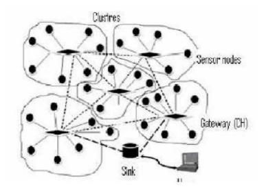
Figure 1. Three Level WSNGs Architecture
