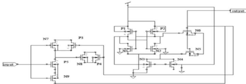
Figure 3: (a) Schematic diagram for 8T with Domino Logic
