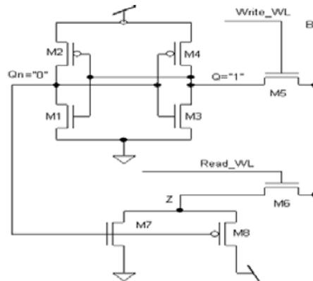
Figure 1: 8T SRAM Design
