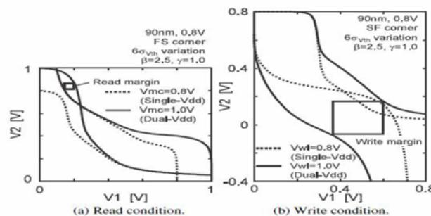
Figure 2: (b) Read and write condition
