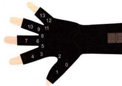
Figure 2. Sensor mappings for 5DT data glove14 ultra
