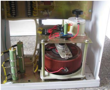
Fig.8.300 volt span variac / 20 amp current rating, sweep 360 degree and motorosed. 230 volt servo motor
