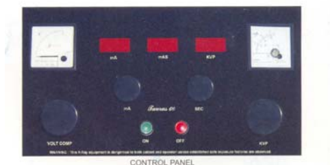
Fig.4. Rotary switch control panel of X-ray Machine
