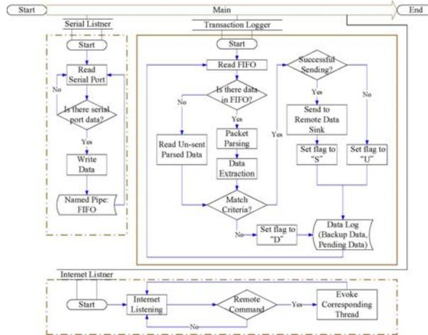
Figure 3: Flowchart of data processing in the gateway
