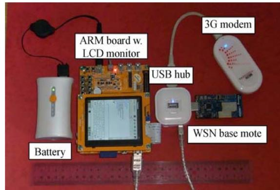
Figure 2: ARM-based gateway devices for simulation.
