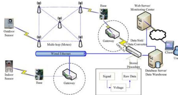
Figure 1: Infrastructure of the WSN Gateway Model for Environmental Monitoring
