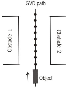
Figure 1. Obstacle collision free path
