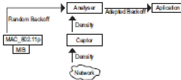
Figure 2: Proposed Mechanism
