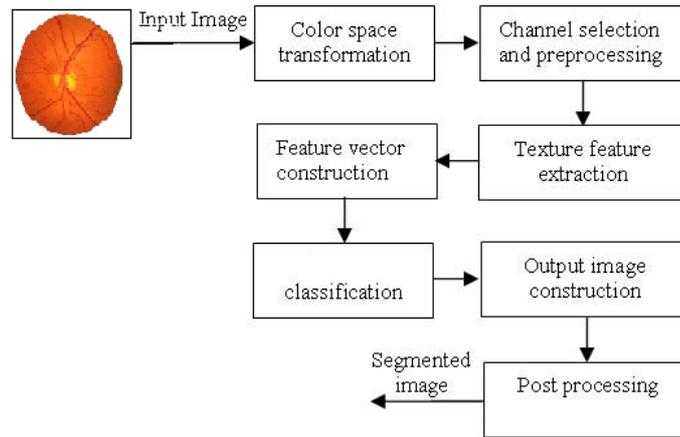
Figure 4: Flow Diagram for the Proposed Segmentation Algorithm.
