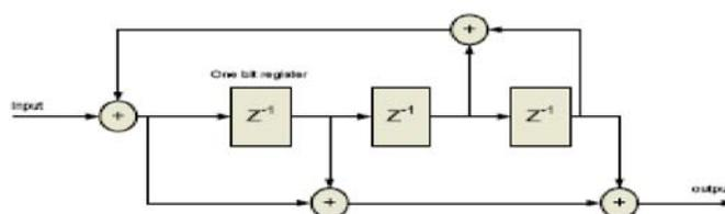
Figure1. Recursive systematic convolution encoder circuit
