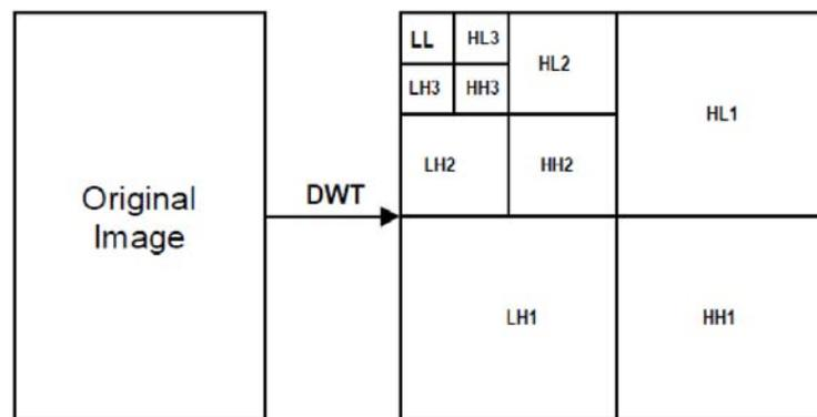
Figure 4: Work Flow of DWT Transformation
