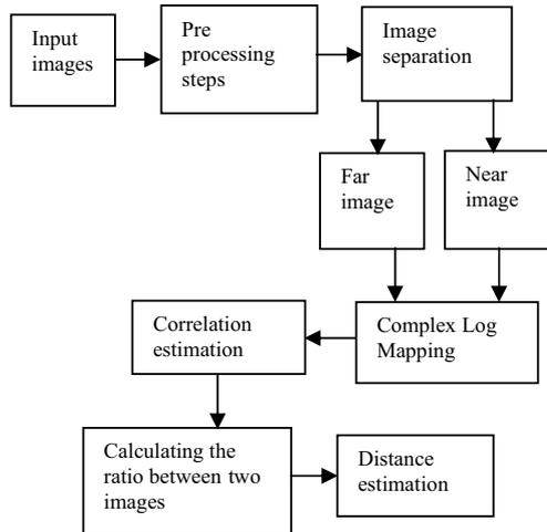
Figure 8. Detailed Block diagram
