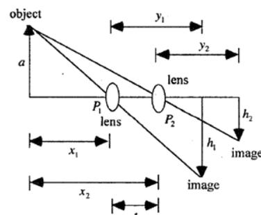
Figure 1. Principle of Distance Measurement
