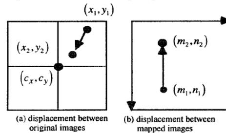
**Figure 7. Displacement Between Corresponding Points**
