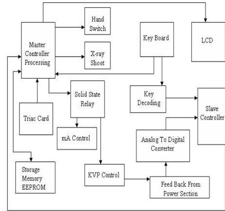
**Fig.6. Block diagram of Digital X-ray Machine**
