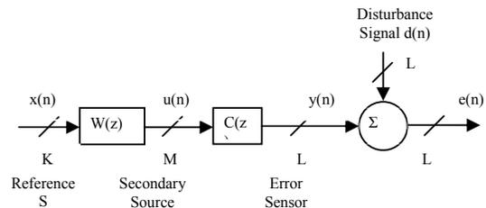
**Fig 1-Multichannel Active Noise Control System**
