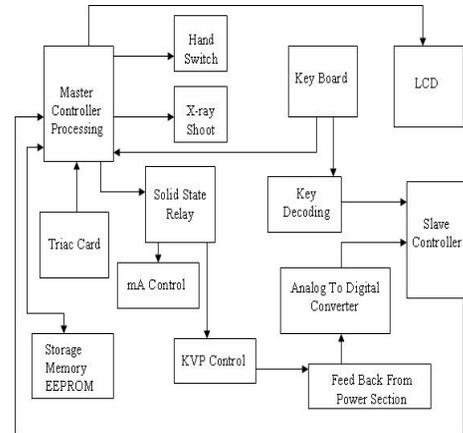
**Fig.6. Block diagram of Digital X-ray Machine**
