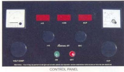
**Fig.4. Rotary switch control panel of X-ray Machine**
