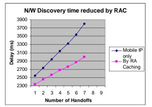
Figure 3. Latency time reduced by RA Caching.
